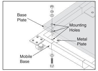
Figure 23. Mounting base plate to mobile base.
